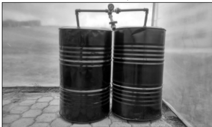
Figure 5 Formation of biogas by the discontinuous system
